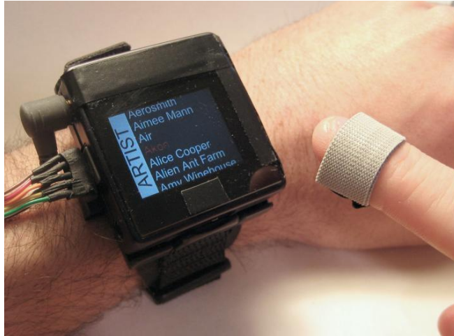
Figure 13. Abracadabra, wristwatch controlled by magnets on fingertips [64].
