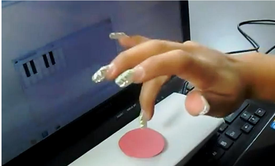
Figure 29. Twinkle Nails, non-contact piano playing
