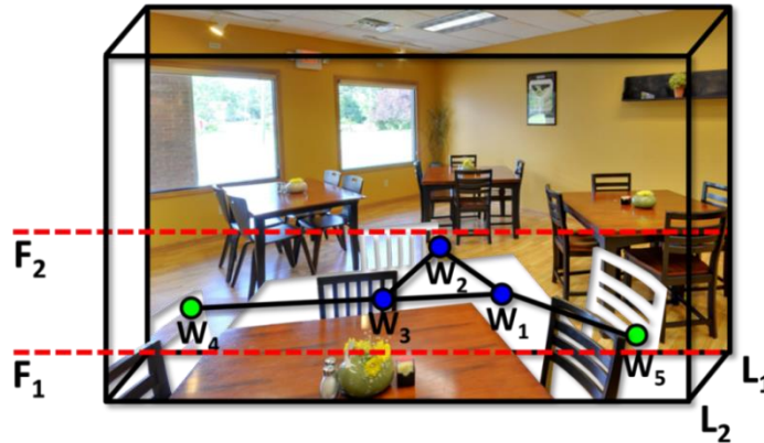
Figure 5.21: Location with 5 waypoints ( W_1 , W_2 , W_3 , W_4 and W_5 ). The front line F_1 and the far line F_2 delimit the region for waypoints.
