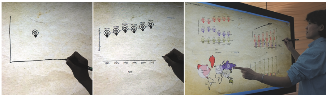
Figure 8.5: Telling a story using SketchStory: (left) A presenter sketches out an example icon and chart axis, (middle) Upon recognition of the chart axis, SketchStory completes the chart with underlying data by synthesizing from example sketches, and (right) The presenter interacts with the charts.
