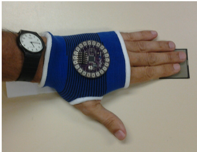
Figure 21 - Force Sensitive Resistor to sense palpation pattern
