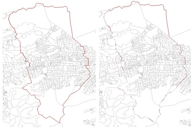
Figure 5.1: Overlaying the maps: evidence of the boundary differences ( slivers ): DP boundaries over census sectors boundaries (left); Census sectors boundaries over DP boundaries (right).
