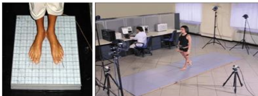
Figure 3 Force platform (left) 2 and a set of high-precision 3D cameras (right). Both instruments are used for estimating center of pressure and center of mass displacements.
