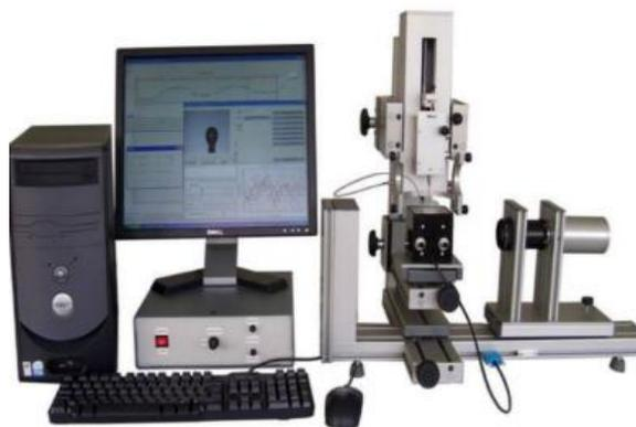
Figura 36 – Tensiômetro Tracker TECLIS.
