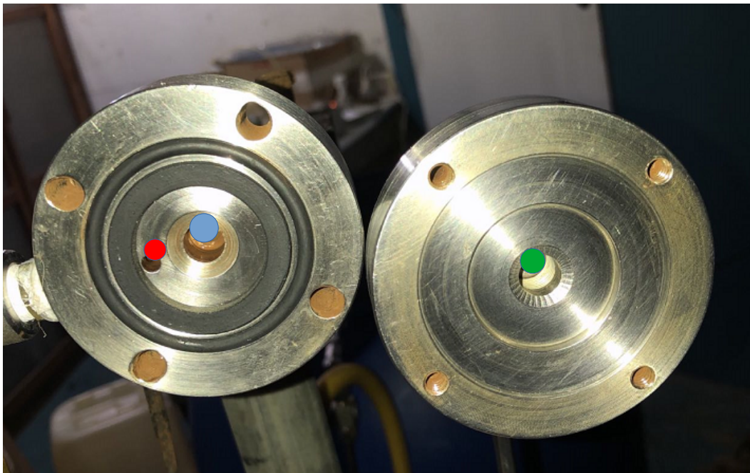
Figure 15: Cross-flow membrane cell. Water goes into the membrane cell from the blue point and goes back to tank through the red point. The filtered water goes out the system from green point.
