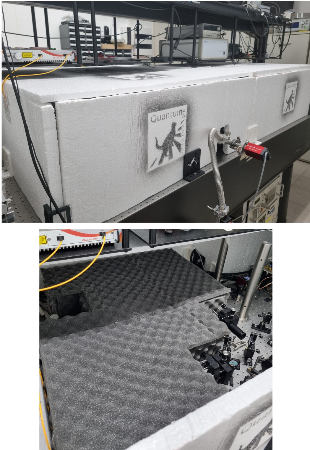
Figure C.2: Experimental insulating case. We have assembled two boxes for thermal and mechanical environment insulation. The external box, shown at the top, is made of polystyrene, while the internal box, shown at the bottom and made of rock wool, encases fiber optics exclusively.
